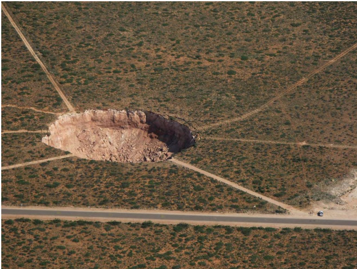
Figure 4-175 JWS sinkhole in northern Eddy County, about three weeks after initial brine well collapse. Pickup truck in lower right corner for scale.
