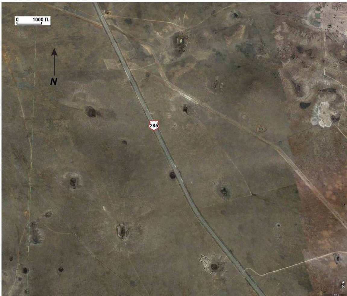
Figure 4-167 Sinkholes along US Highway 285 corridor, about 30 miles southeast of Vaughn, NM
